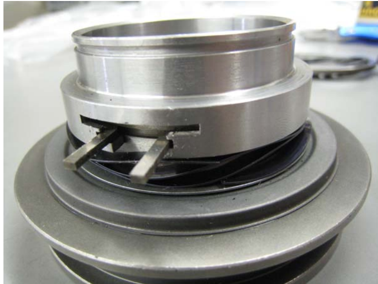
Retaining Clip shown latched into the closed position.
