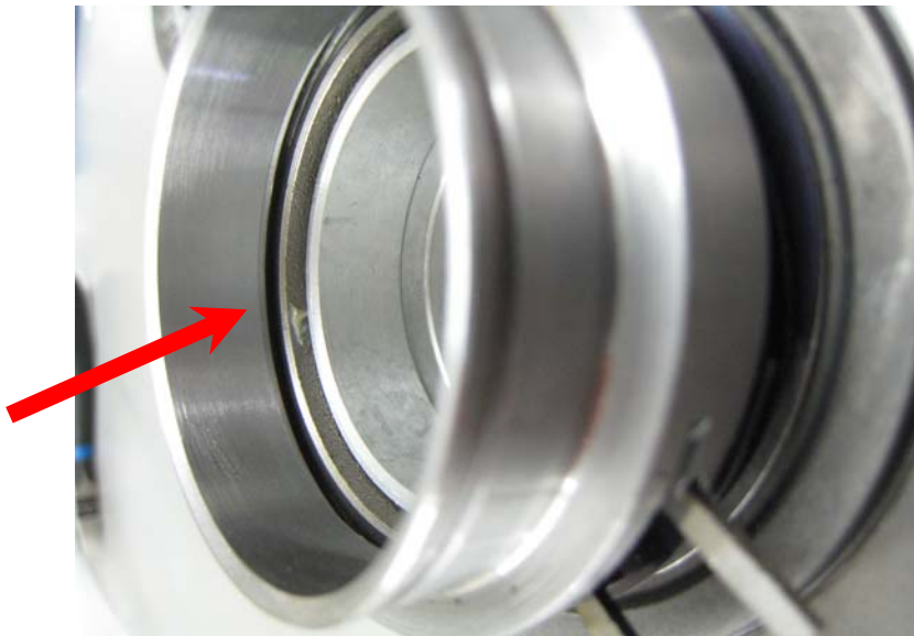
The internal groove for the Spiral ring is clearly visible between the adapter (closest to camera) and the Clutch Release Bearing.
