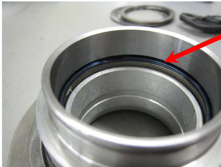
Completed installation of the Spiral retaining ring
