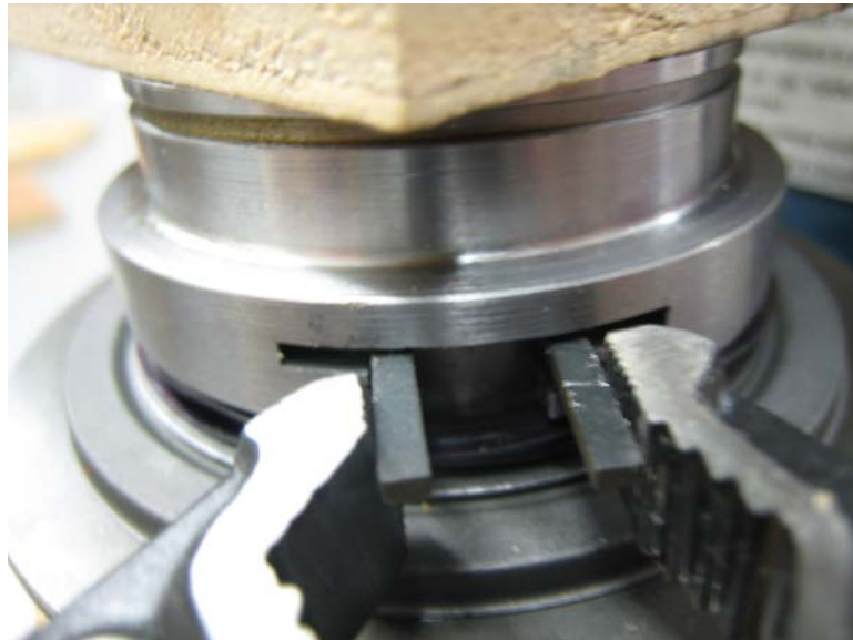
Retaining ring in compressed position so ears will pass between fingers.
