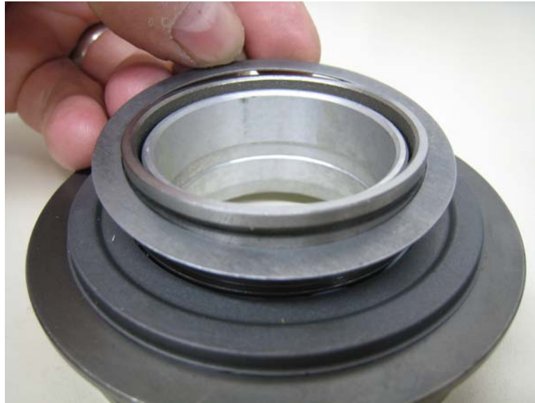
Original shim placed onto the Porsche Clutch Release Bearing first
