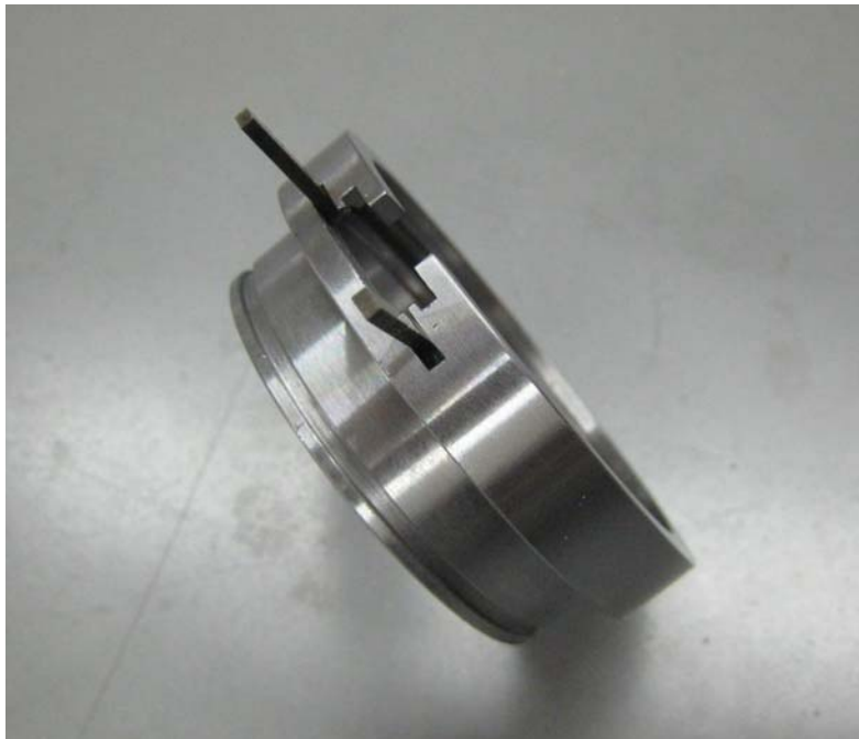
AP Racing adapter for the O.E. Porsche Clutch Release Bearing.
