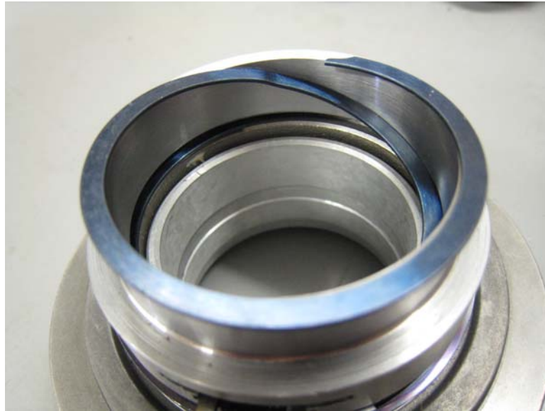
Installing the Spiral retaining ring
