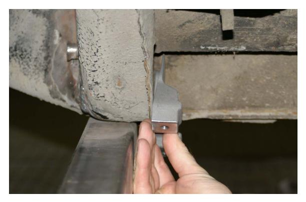
Cut a strip of material 2 - 3 mm (.080" - .125") thick and ~ 10mm (3/8"ths) wide. Bend this to match the perimeter shape of the "tombstone" section of the RARB console. Weld this material perpendicular to the mount so that you have a flange extending laterally to close the gap between the RARB console and the chassis box section.
