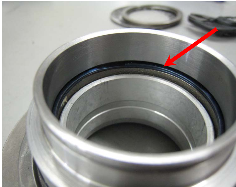
Completed installation of the Spiral retaining ring
