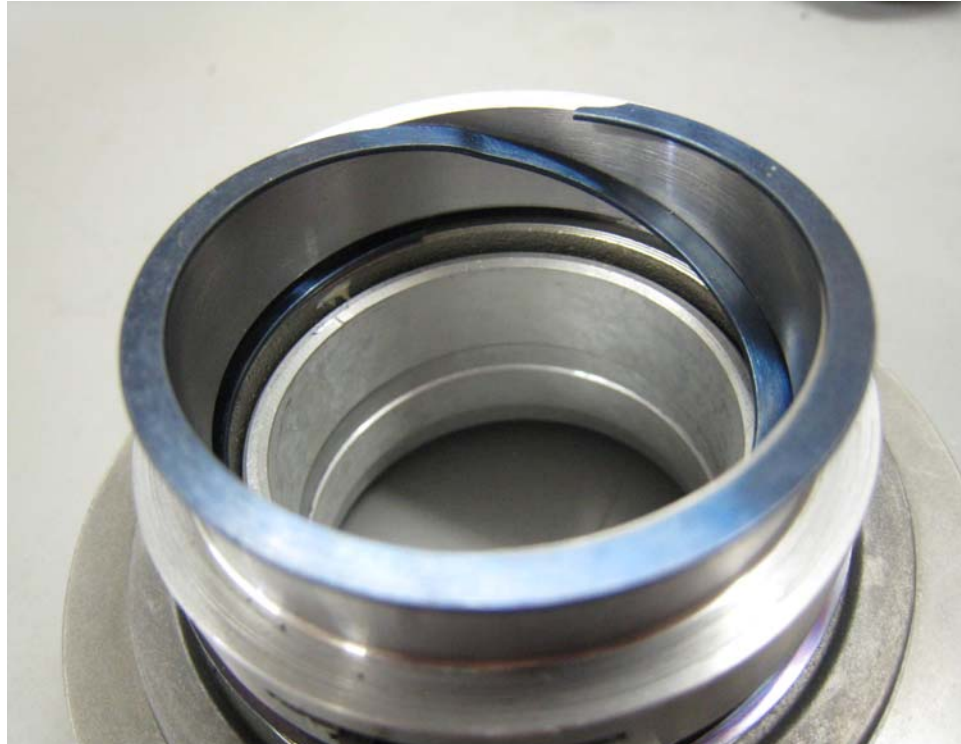
Installing the Spiral retaining ring
