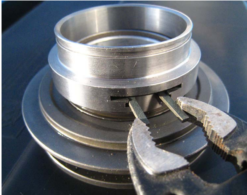
Retaining ring in compressed position so ears will pass between fingers.
